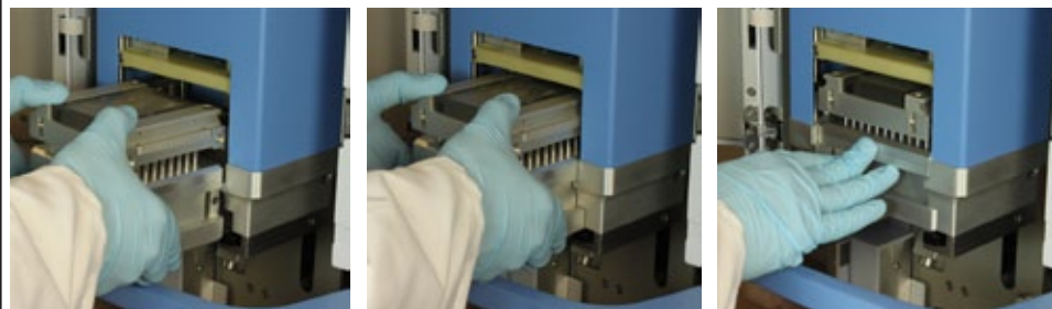
Pipetting head loading into NTC pipetting module
