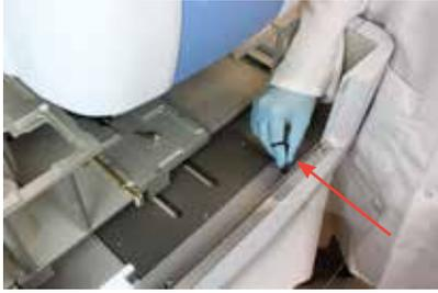
5. Hold the front of the stage with one hand, and with the other reach back underneath the stage and slide the locking pin toward the front of the unit to engage it under the stage.
