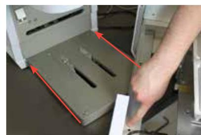
4. Secure the stage assembly onto the base unit with the four button head screws using a 4 mm Allen wrench.
