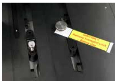
2. Manually slide the stage locking pin to the rear of the base unit.
