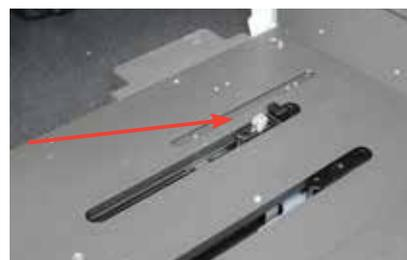
3. Carefully place the stage assembly onto the base platform and align to the four corner pins. Push gently, but firmly, onto the stage so it drops down onto the four pins and locks into position.
