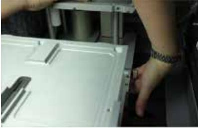
6. Install connectors (stage control cable/shield cable) to the tower. Also connect the tubing and tip wash sensor into the pump module using a 2.5 mm Allen wrench.
