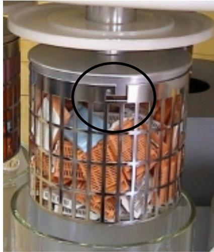
The baskets are held in position by a **four point** bayonet connector.
