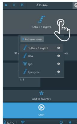
Built-in protein protocols allow you to select between four different protein types or create your own. Measure using the  $\mu$ Drop Plate, microplate, or cuvette, and view your concentration and purity results.
