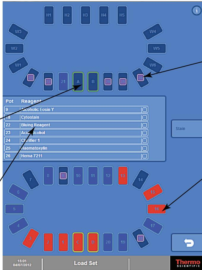
The layout shows the upper and lower levels, along with the pots and a list of the required reagents.
