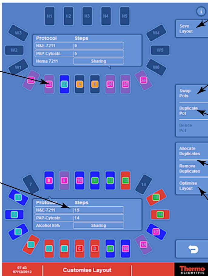
The number in the pot identifies its position within the instrument.
