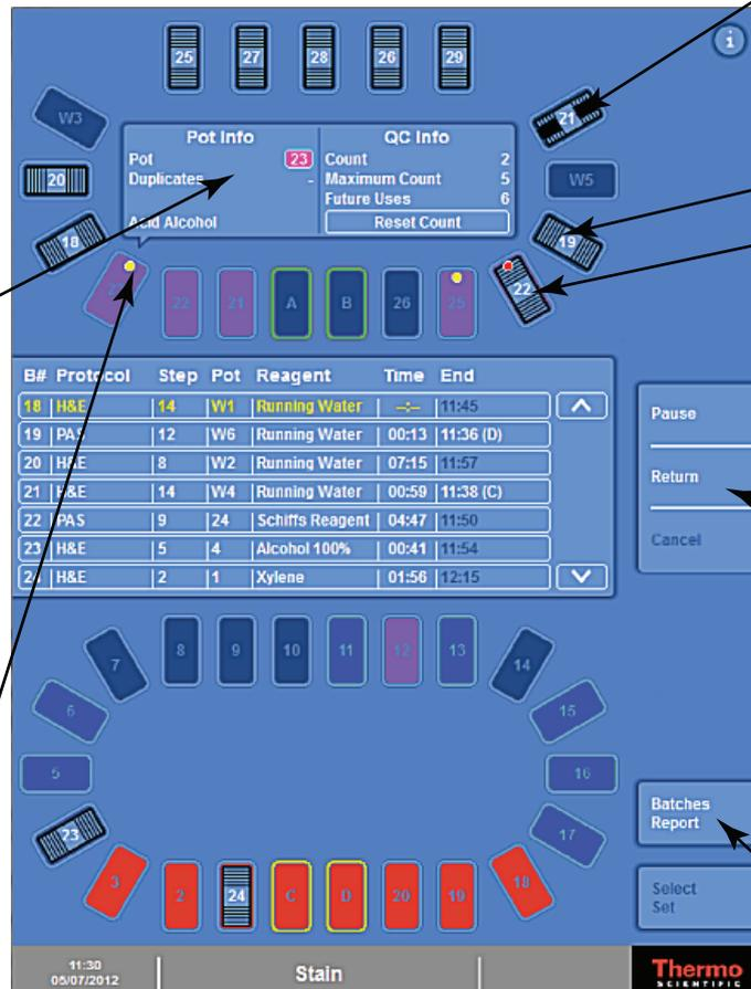
Amber QC alert displayed when reagent is within 3 uses of its limit. Red QC alert displayed when limit is reached or exceeded.
