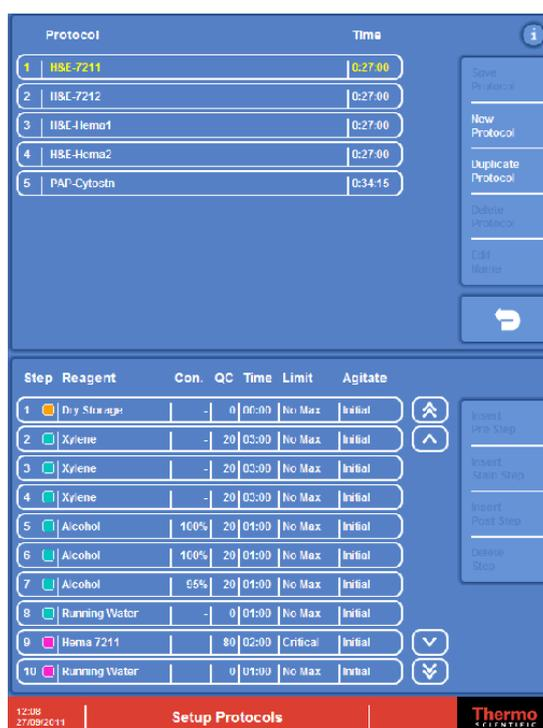
The screenshot shows the 'Setup Protocols' screen. The top panel displays a list of protocols with columns for 'Protocol' and 'Time'. The bottom panel displays a detailed view of a protocol's steps with columns for 'Step', 'Reagent', 'Con.', 'QC', 'Time', 'Limit', and 'Agitate'. The steps are color-coded according to the table above.
