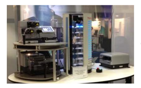
Thermo Scientific Orbitor RS plate mover with BioTek's 405 washer, MultiFlo dispenser and Epoch reader makes a versatile bench top automated workstation.
