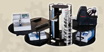
↑ The Thermo Scientific Orbitor RS can access complicated set-ups, including stacked instruments, as well as reach virtually any benchtop instrument. It also fits comfortably in most biosafety cabinets.
