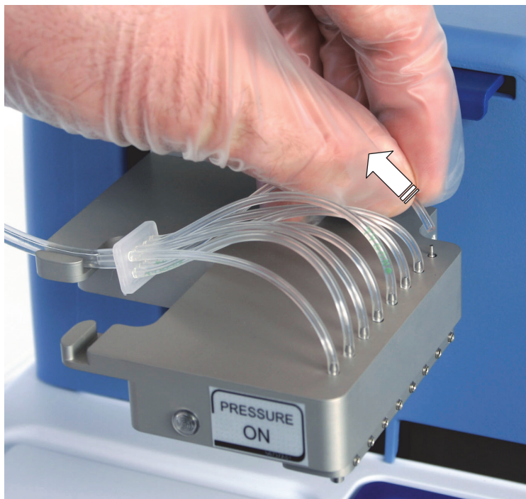
Figure 5–25. Detaching a dispensing valve tube end
