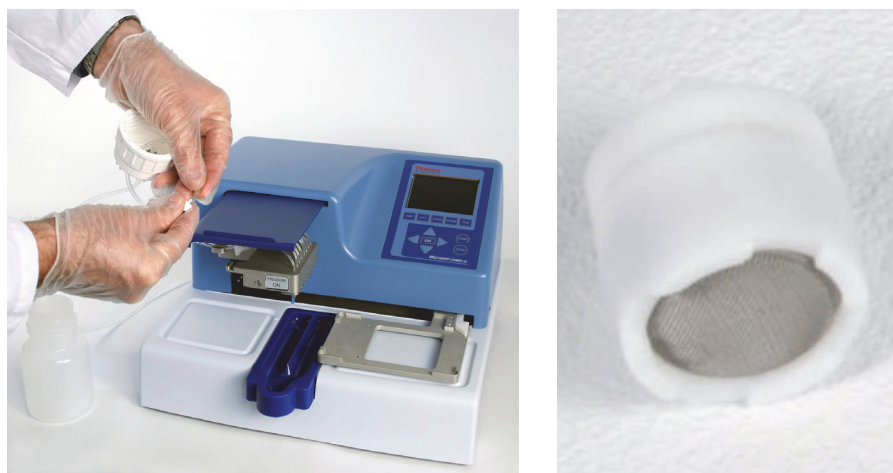
Figure 4-18. Removing the reagent filter
