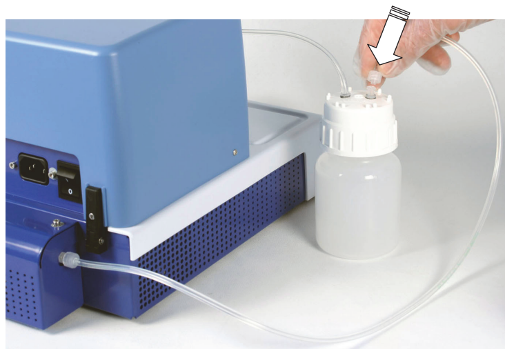
Figure 3-11. Connecting the hosing to the reagent reservoir
