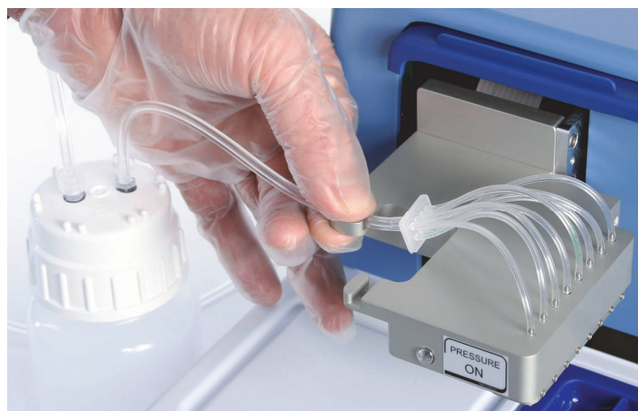
Figure 5–31. Replacing the tubing set and manifold
