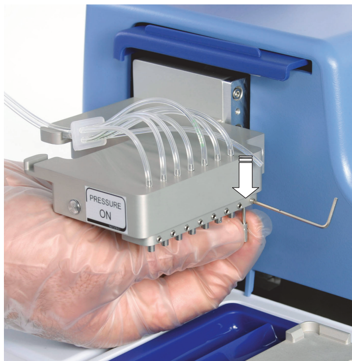
Figure 5–29. Pulling the dispensing valve downwards
