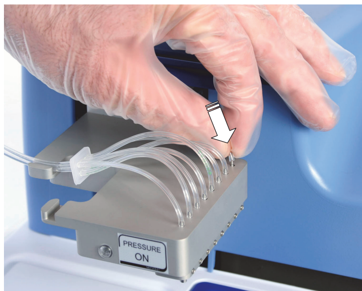
Figure 5–26. Reconnecting a dispensing valve tube end
