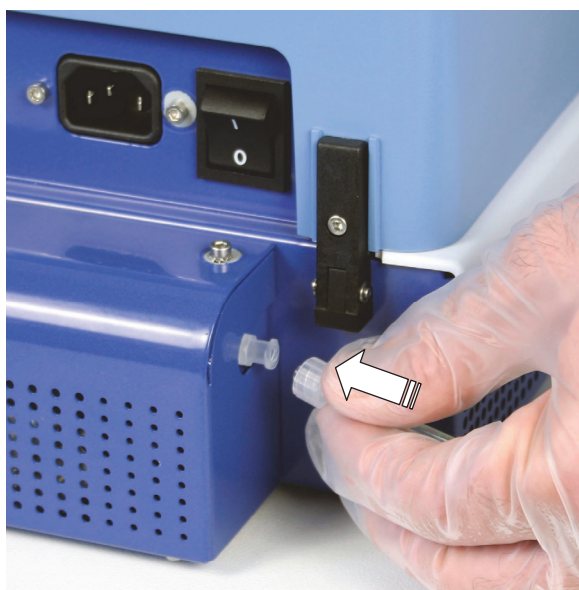
Figure 3–10. Connecting the hosing to the pressure/vacuum system
