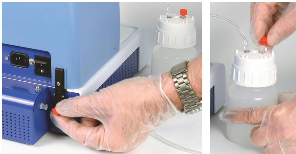
Figure 3–9. Removing the red luer plugs
