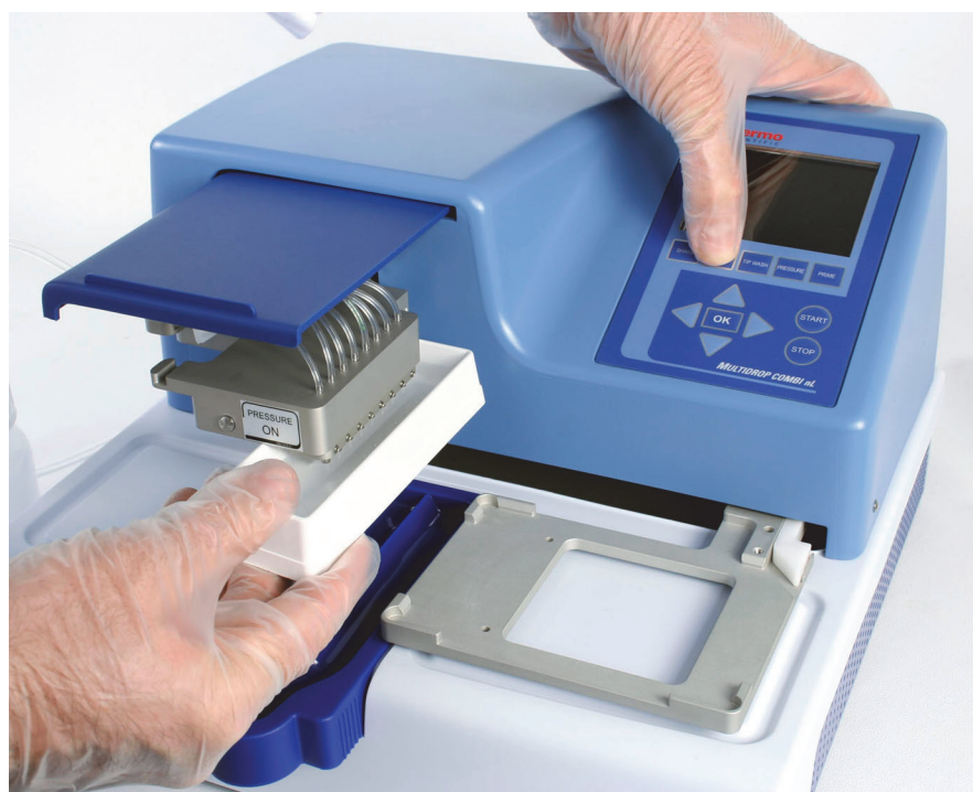
Figure 5–24. Cleaning the tubings using a reagent basin
