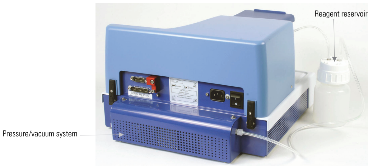
Figure 4–17. Reagent reservoir connected
