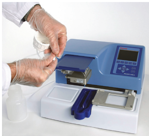
Figure 5–23. Removing the reagent filter
