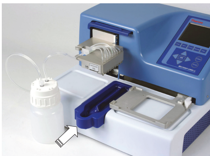
Figure 3–8. Inserting the priming vessel
