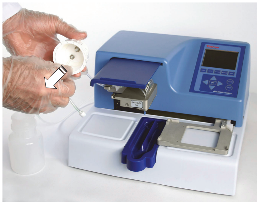
Figure 5–27. Removing the reagent filter with tube
