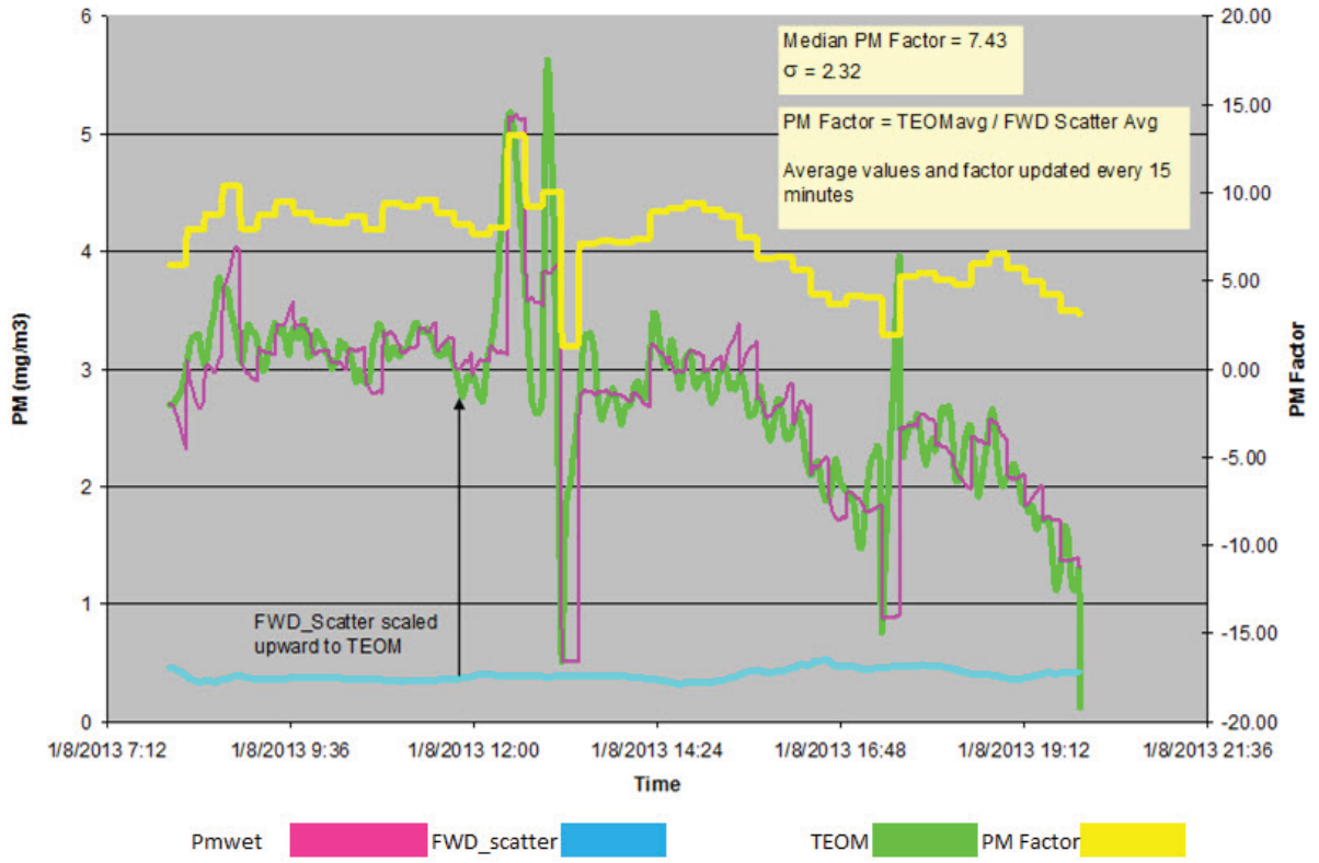
Figure 5: LSS scattering responses from Alpha test. PM Factor is updated every 15 minutes. Forward scatter is continuously scaled to TEOM.
