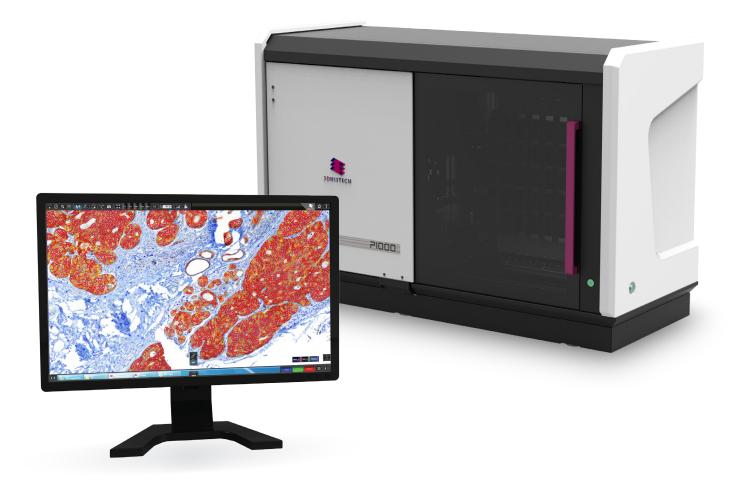
Thanks to its unprecedented capacity and unparalleled speed, PANNORAMIC<sup>®</sup> 1000 offers automated, "walk away" slide scanning for a whole day's scanning needs, speeding up the workflow and freeing up valuable lab resources for other important tasks.
