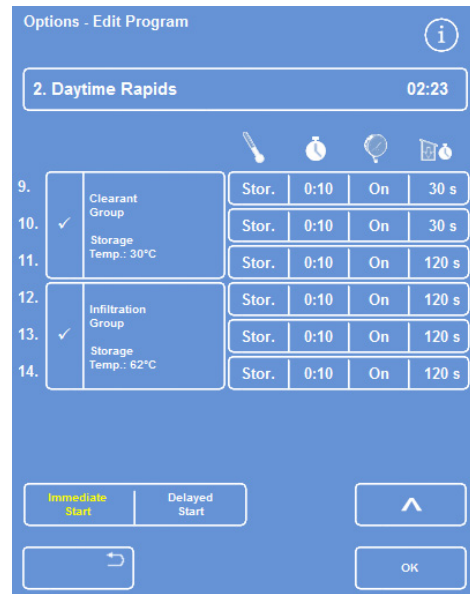
Clearant and infiltrant step details
