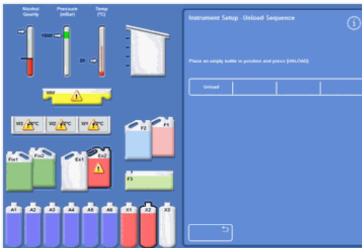
Unloading clearants – Ex2 full and X2 outlined
