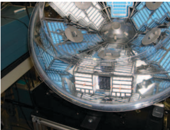
Figure 4 Rack and Cassette in RTP Processor
